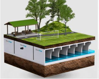
FIGURE 3.4.2: Rendered view of subsurface water detention vaults
