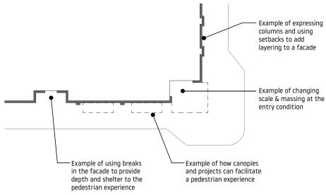
FIGURE 4.2.2: Example of facade setbacks and articulation.
