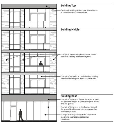
FIGURE 4.2.1: Example of successful building material composition.
