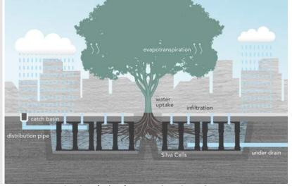
FIGURE 3.4.3: Section view of subsurface water detention vaults
